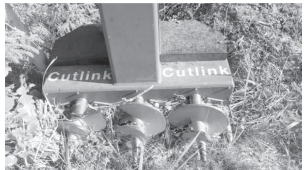
**Fig. 2** Cutlink device based on rotating cone-shaped shears that cut 50–100 cm wide corridors between and around seedlings
