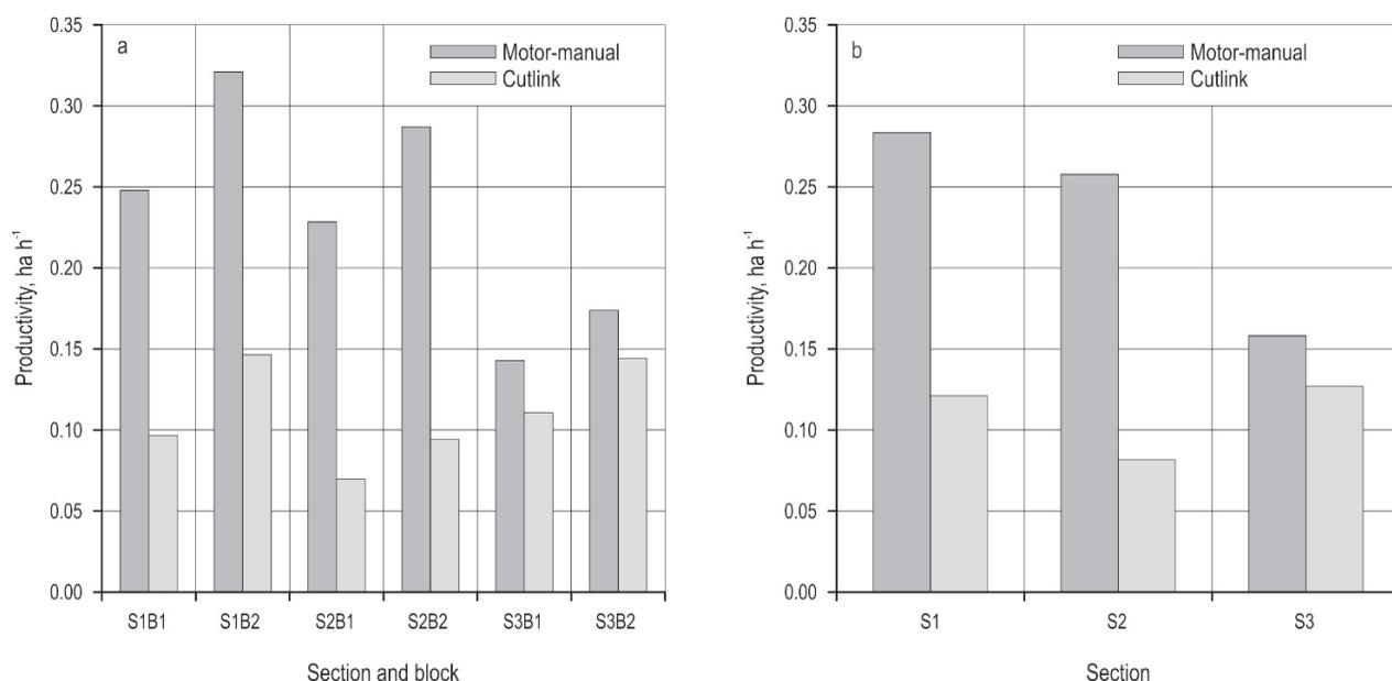
**Fig. 3** Productivity (ha h<sup>-1</sup>) of motor-manual tending and Cutlink device in each block (a) and average of each section (b)
